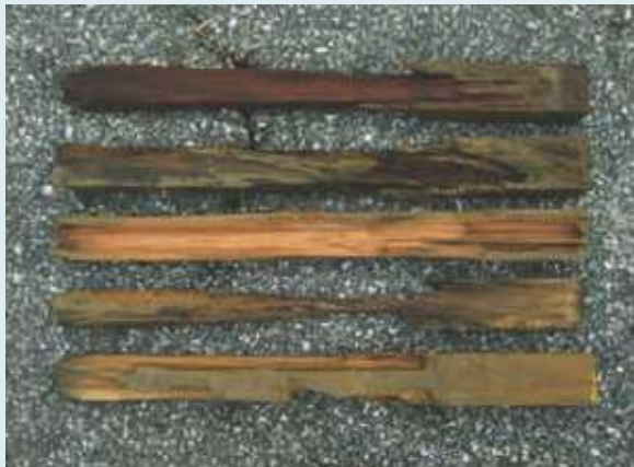
Beberapa sampel kayu yang diserang anai-anai Some of the wood samples were attacked by termites
