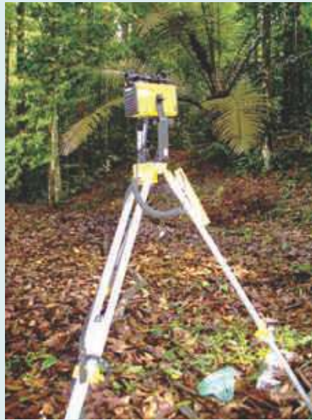
Alat Hand Held Laser Criterion boleh mengukur diameter dan tinggi pokok dari lantai hutan A Hand Held Laser Criterion device used for measuring diameter and length of trees from the ground
