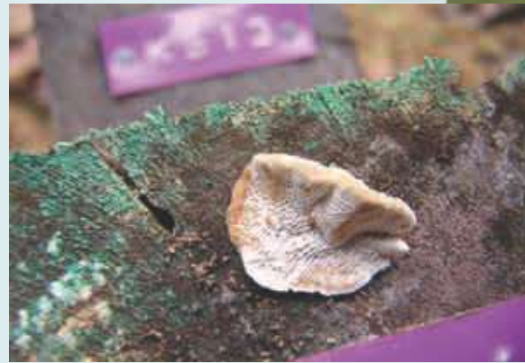
Kandul spora kulat pereput kayu di atas sampel kayu yang terdedah Fruiting body of wood decaying fungus on exposed wood sample
