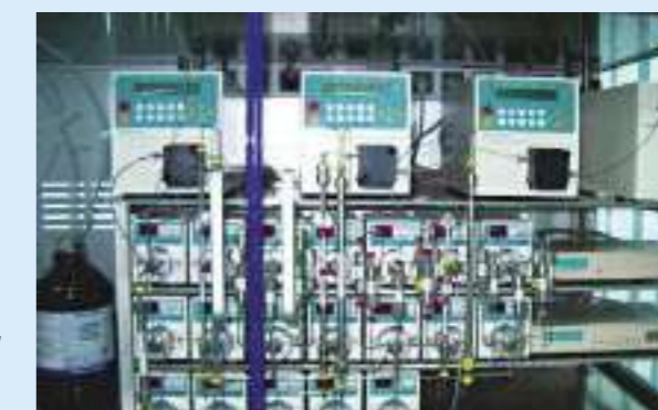
Alat SEP BOX mengasingkan ekstrak tumbuhan ubatan kepada sebatian The SEP BOX equipment separates medicinal plant extracts into their constituents
