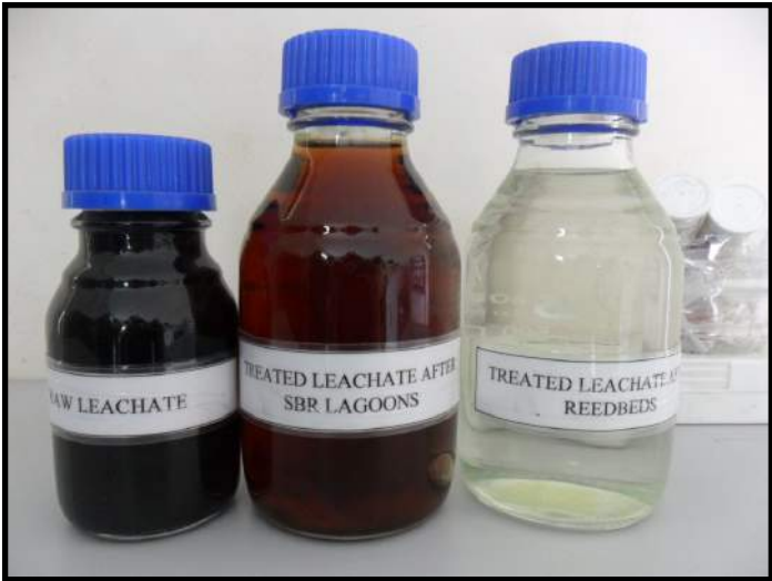
Comparison between the raw leachate and treated leachate with Reedbeds
