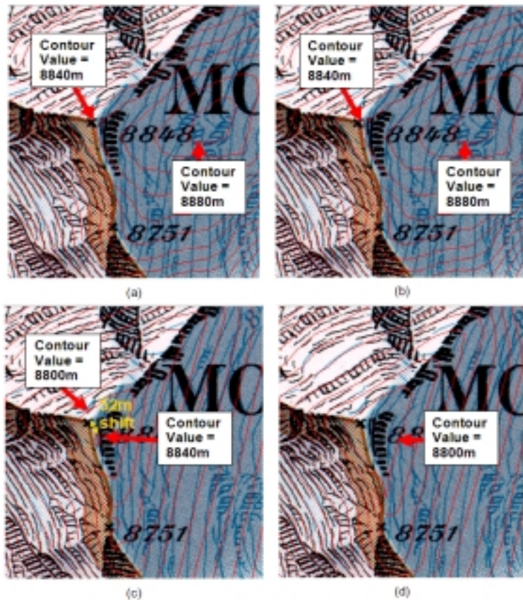
Figure 10: Result on plainimetry and height value on Mount Everest using single model (model 5409_5410) (a) DTM25 (b) DTM50 (c) DTM25Br (d) DTM50Br
