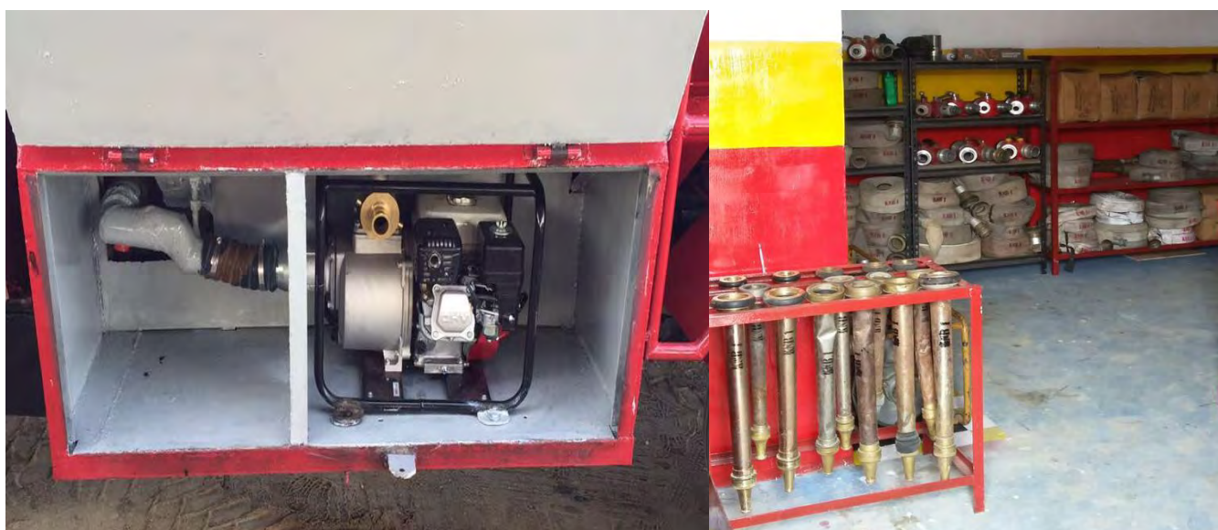
Water tanks equipped with water pumps, high pressure hoses with nozzles
