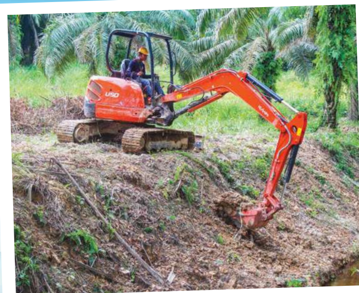
Mini excavators, that are used in Leepang A Estate, are one of the mechanisation tools used to clear terraces, improve road conditions as well as speed up harvesting operations.
