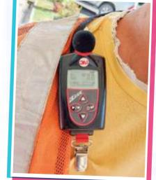
The workers wore the personal noise dosimeter. for eight hours in order to determine their evel of noise exposure as they worked.
