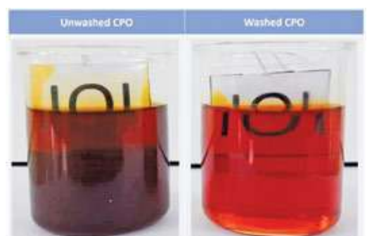
Look at how the CPO washing dilutes the inorganic chlorides.
