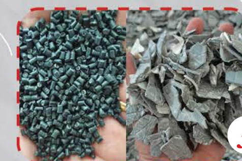
The used filter plates are segregated by grade before being crushed into smaller particles of below 25 mm.
