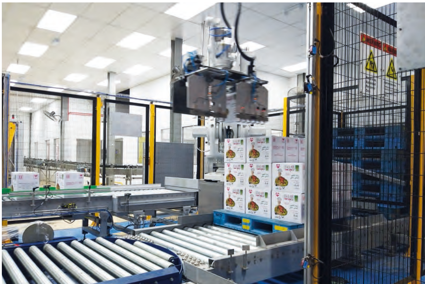
The fully-automated consumer pack filling line at IOI Pan-Century Edible Oils Sdn Bhd enhances production efficiency.
