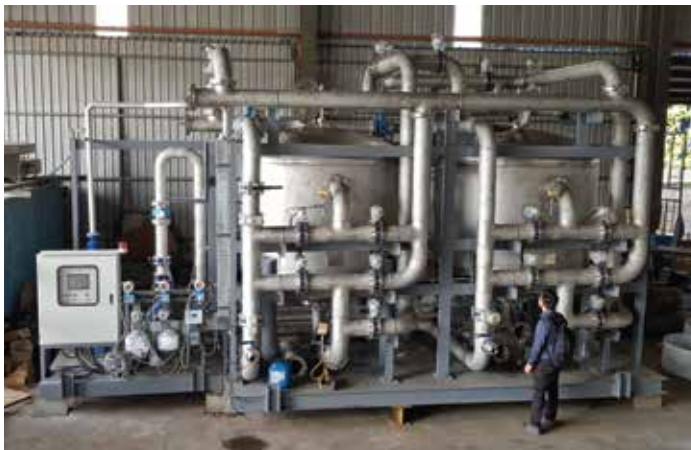
150 m 3 /hr, Auto Operated fully SS304 Multimedia filter.
