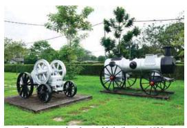
Concrete crusher & portable boiler circa 1930s
