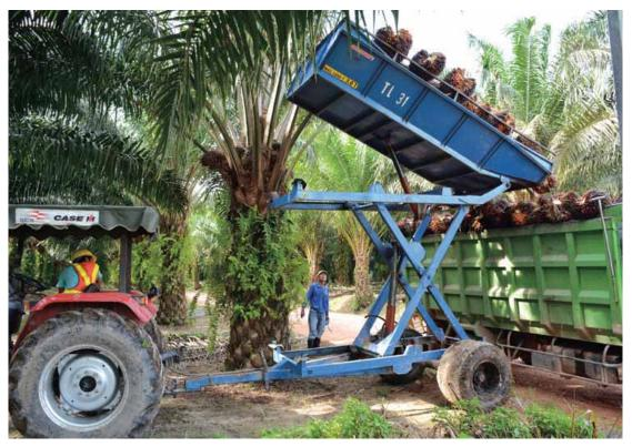
In-field mechanised FFB evacuation done with the Tractor tanker system on our Lada Estate in Central Kalimantan.
