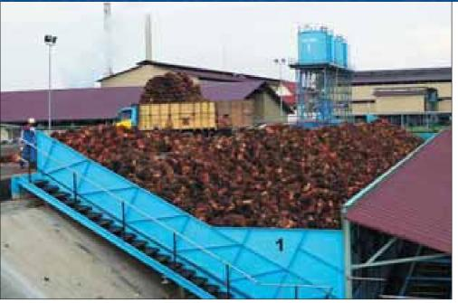
The Lada Mill FFB ramp which can hold up to 700MT of FFB at any one time.
