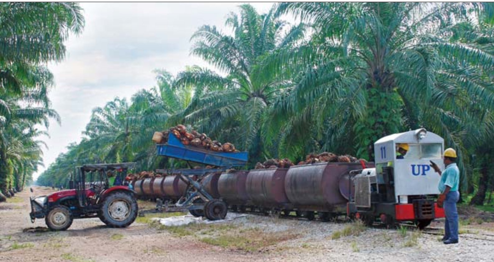
FFB from in-field collection is loaded on to cages which are then pulled by the diesel locomotive. UP's unique light railway system ensures high quality palm oil with the speedy and environmentally friendly transportation to the mills.
