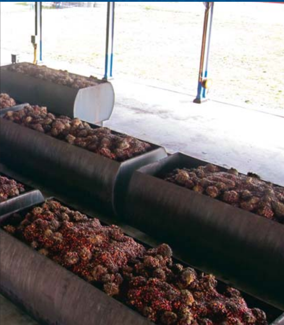
10 MT cages waiting to be charged into the 60 MT sterilizers at the Lada Mill, Central Kalimantan. The Lada Mill has a 180 MT sterilizing capacity.
