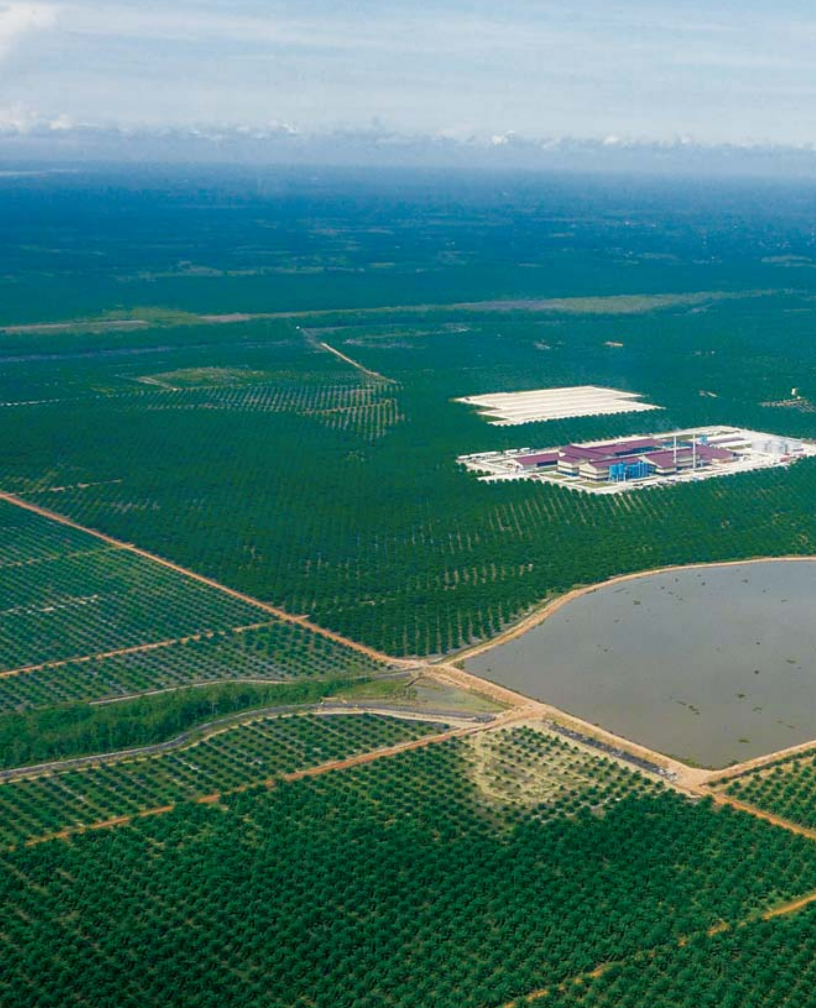
An aerial view of Lada Estate in Central Kalimantan showing the water reservoir with a storage capacity of nearly 2 million cubic meters built to ensure uninterrupted water supply to the mill. Also seen here are the mill and office complexes.
