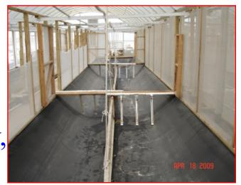
Each RW was equipped with a center longitudinal fiberglass partition positioned over a 5.1 cm PVC pipe with sprayer nozzles
