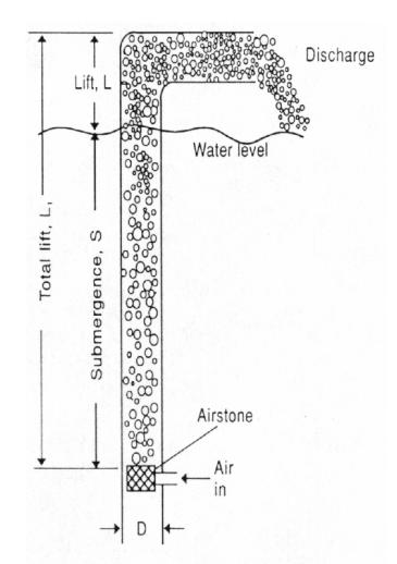
One of the main factor affecting the efficiency of an airlift pump is the submergence of the lift tube
