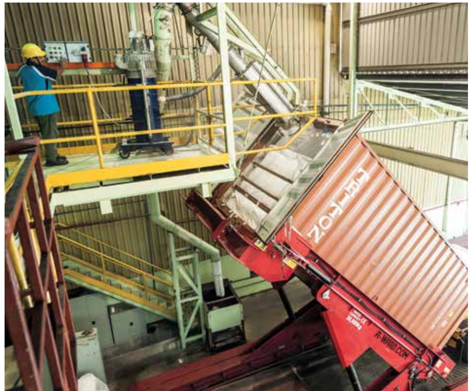
The process of transferring our refined sugar products into the container for delivery.
