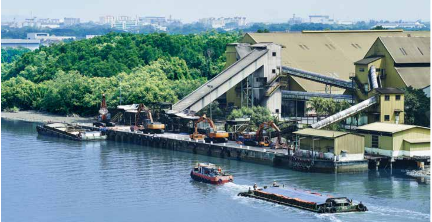
A crane and excavator equipped with grab buckets are used to unload raw sugar.
