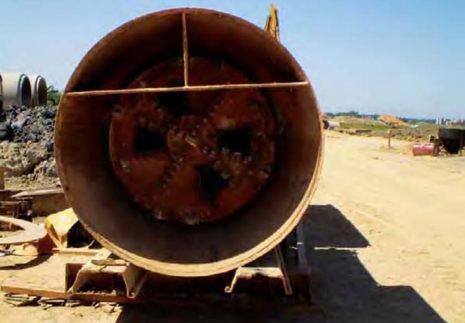
Front view of Pipe Jacking Cutter head 1500mm Diameter for Kota Kinabalu Sewerage works, Phase 1, Sabah
