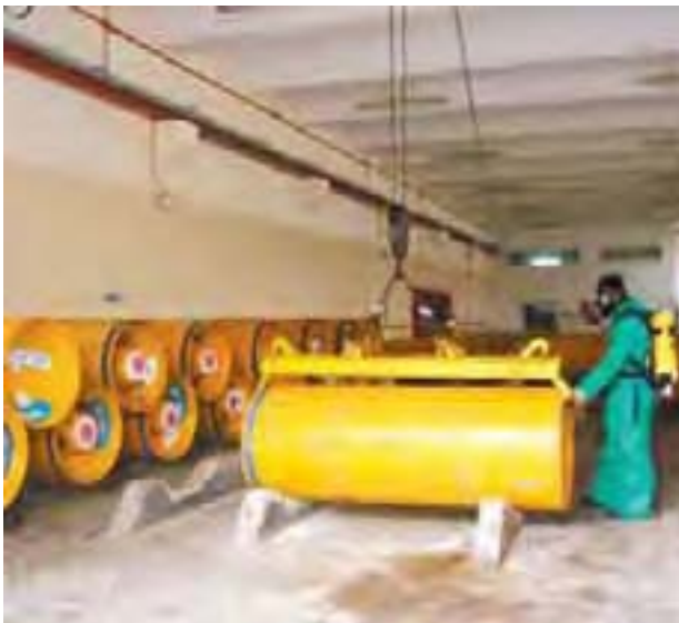
Operator wearing Self Contained Breathing Apparatus during emergency drill situation
