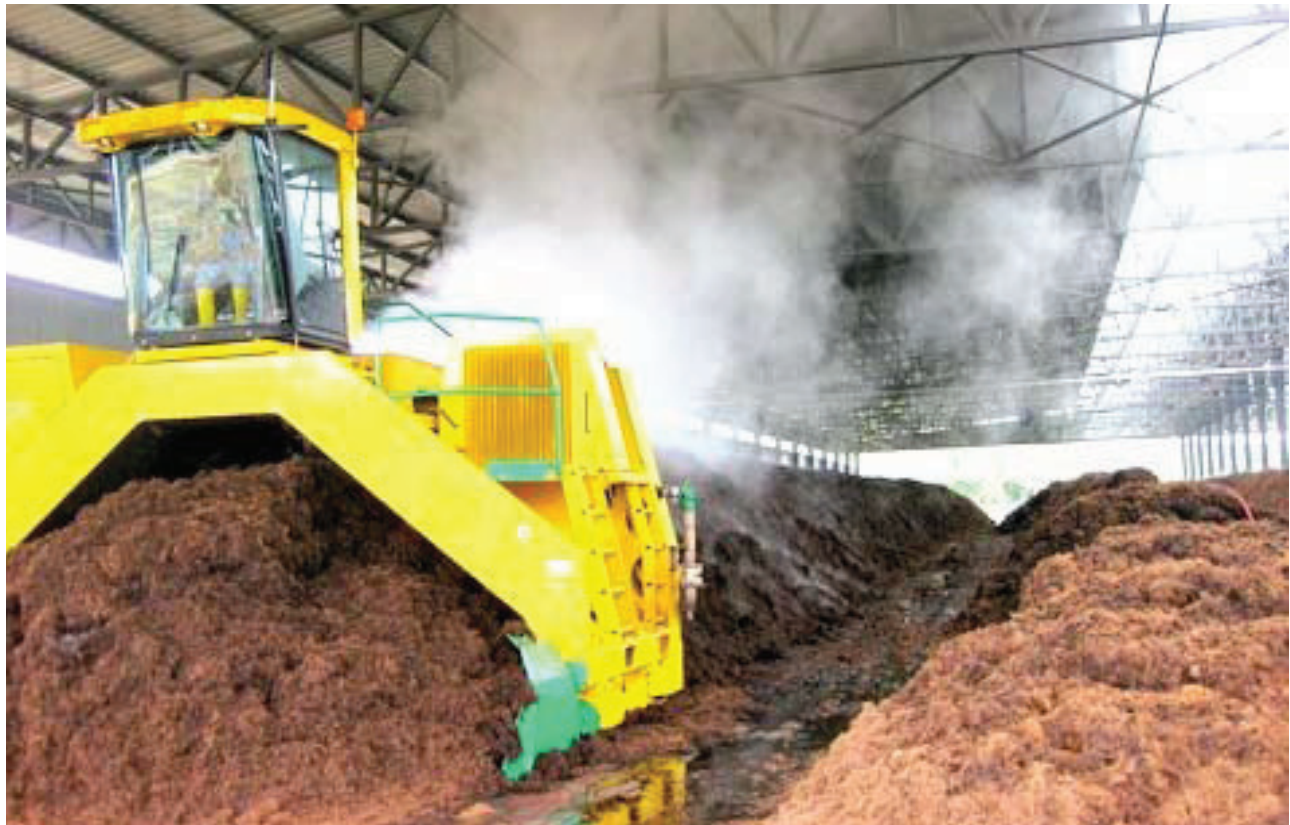
Figure 3. Turning windrows to optimize microstructure, O 2 and moisture content of compost.
