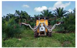
MTG is used to load FFB
