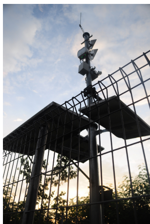
Service pole with telemetric and hydrological equipment; inside a datalogger; rain gauge
