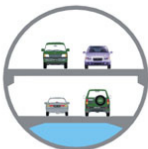
A two-level motorway and a third level for stormwater conveyance Source: JPS
